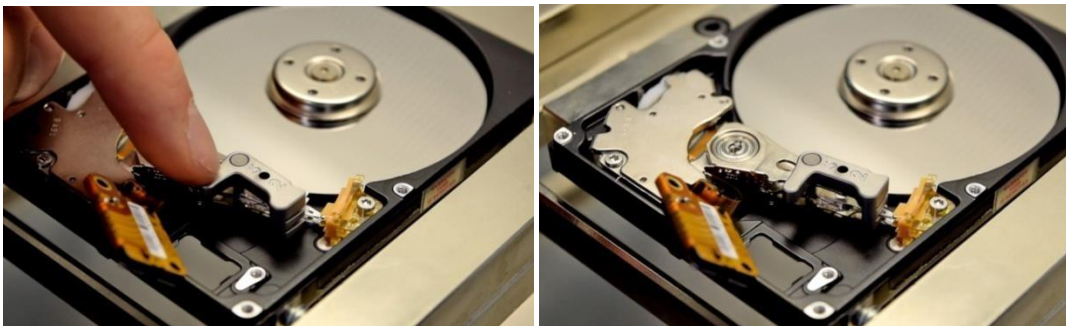
Picture 6.6 Rotating the tool - snouts are positioned between the heads
