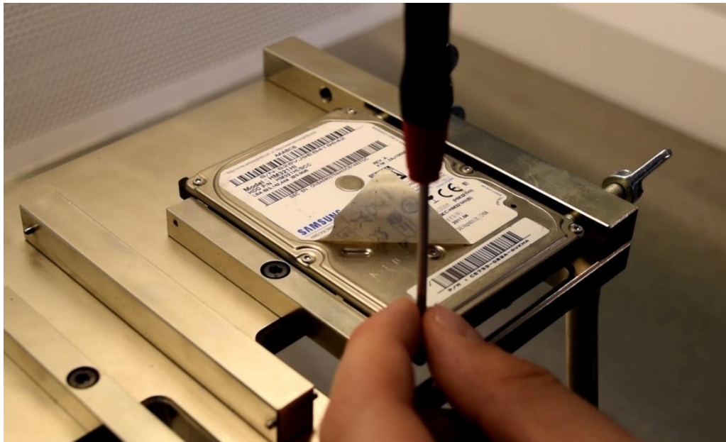
Picture 6.2 Unscrewing the lid
