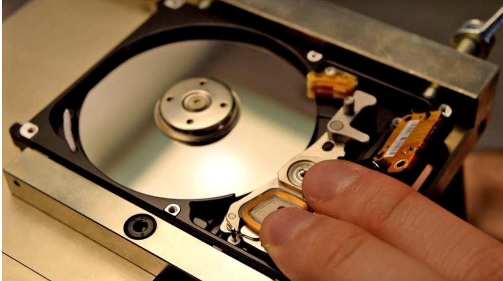
Picture 6.10 Sliding the heads off the donor drive ramp
