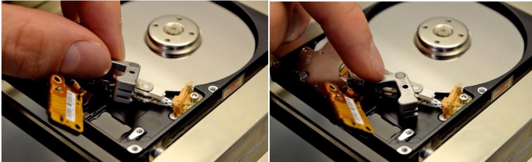
Picture 6.5 Mounting the tool on the actuator arm
