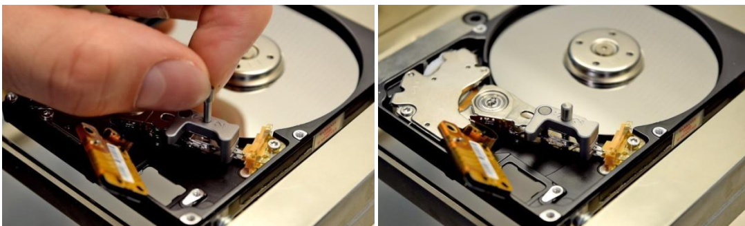
Picture 6.7 Securing the heads with the tool
