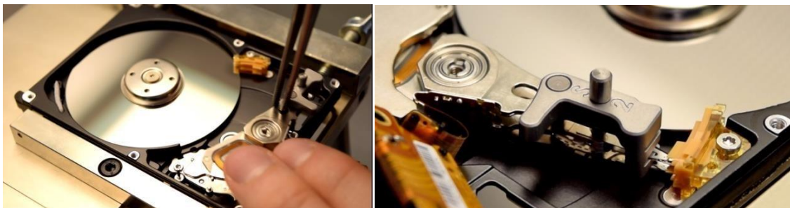
Picture 6.12 Mounting the heads on the patient drive and moving them to the ramp
