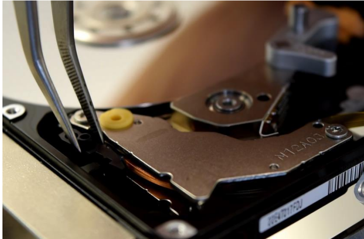
Picture 7.8 Removing the security brake
