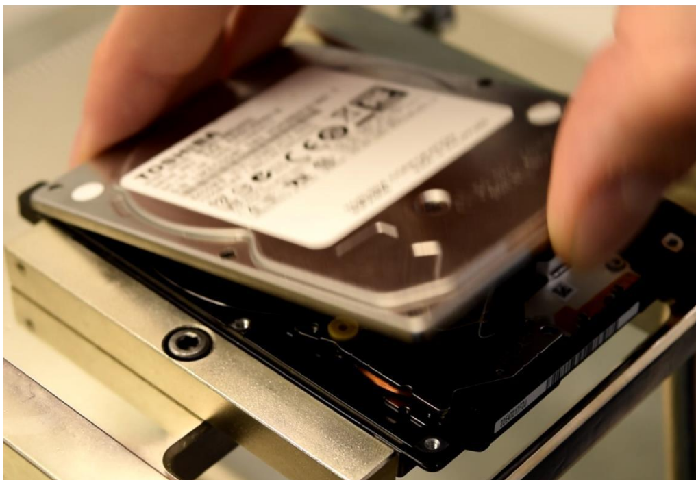
Picture 7.3 Opening the casing
