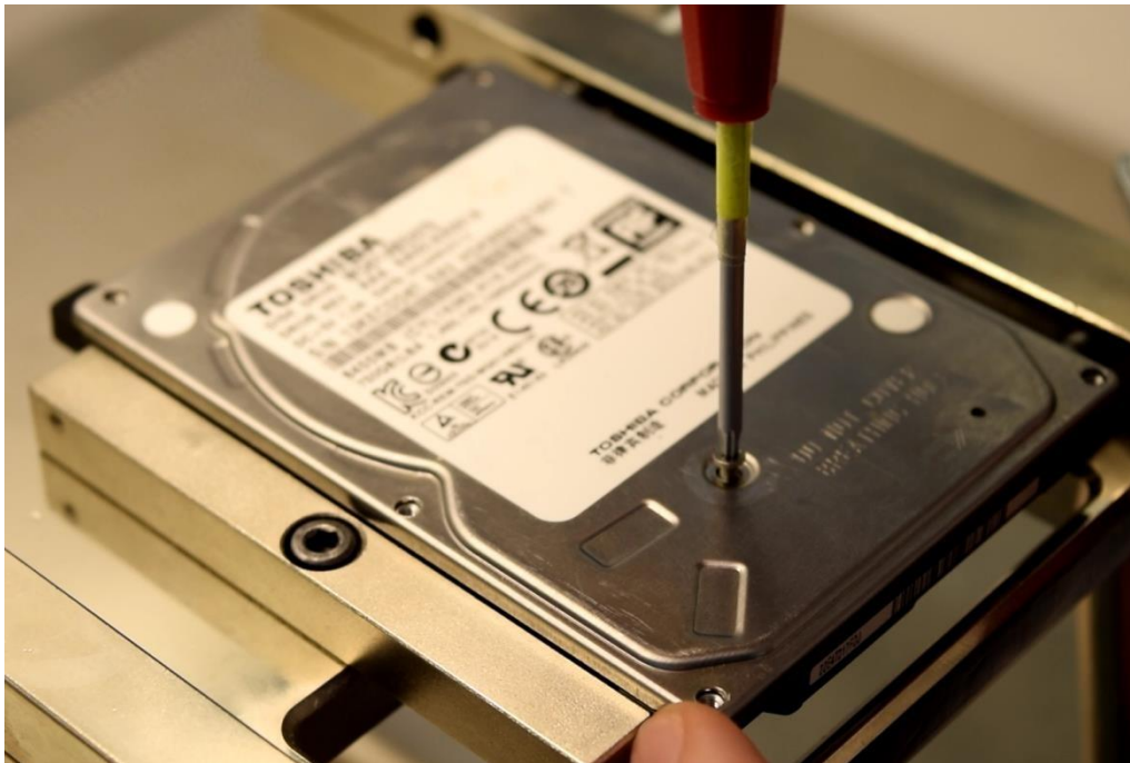
Picture 7.2 Unscrewing the lid
