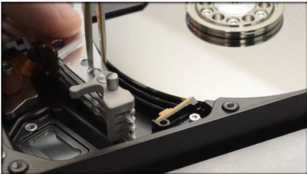
Picture 7 (mounting the heads in a patient drive)
