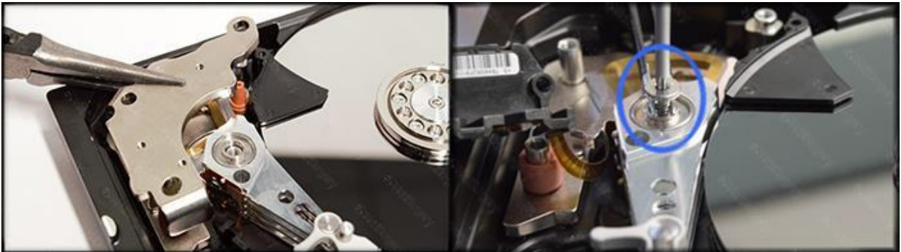
Picture 2 (removing the magnet and securing the head arm with a screw)
