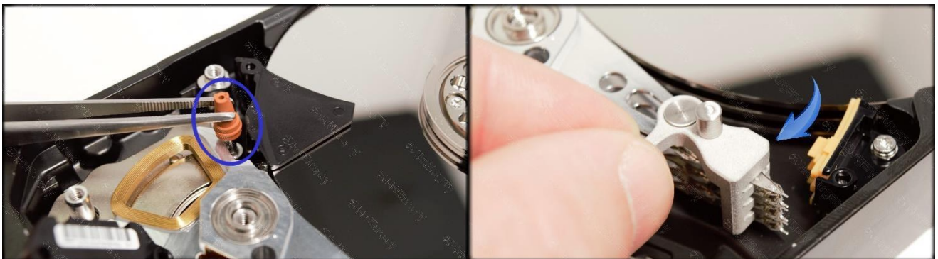
Picture 5 (removing the brake and scrolling the heads off the ramp)
