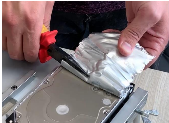
Picture 5.8. Winding the membrane using the pliers
