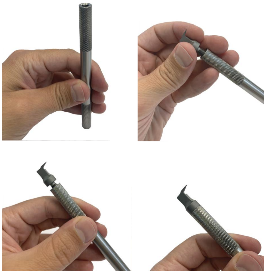
Picture 4.1. HDDS Helium Opener assembling
