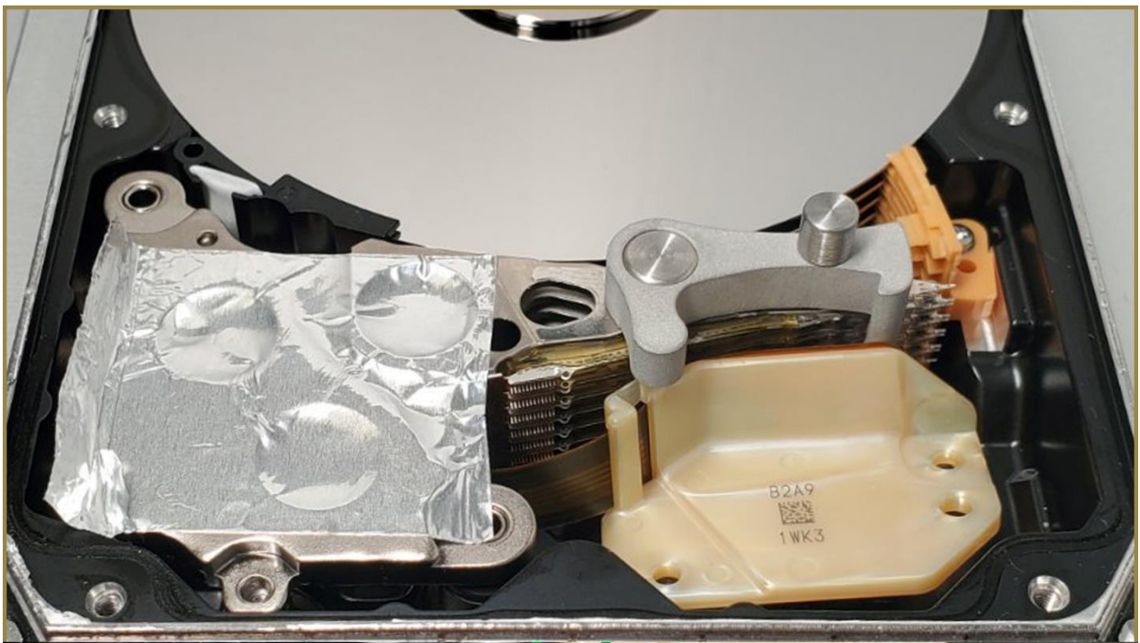
(picture 6 – aluminum tape applied over magnet and HSA)
