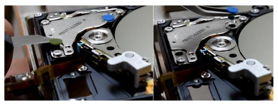
Picture 6.5 (Removing the security brake(s))
