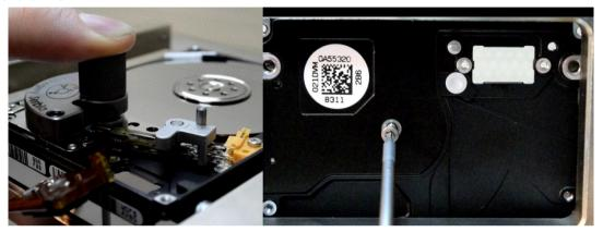
Picture 6.13 (Holding the support tool locknut (left) while loosening the screw that is holding the head arm connected to the casing of donor drive (right))
