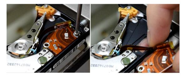
Picture 6.3 (Dismounting the flat cable connector)
