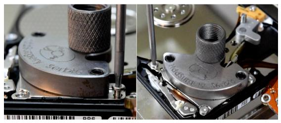
Picture 6.17 (Tightening three screws (fixing magnets to the patient drive casing))
