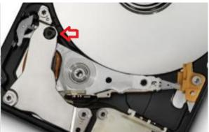
Picture 4.2 (Left - Hitachi 2.5" hard drive with two security brakes on the upper magnet; Right - HDD with one security brake in the upper magnet)
