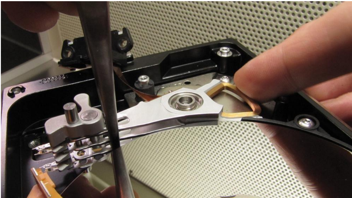
Picture 6. (mounting the heads in a patient drive)
