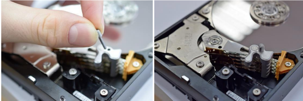
Picture 6.7 Securing the heads with the tool
