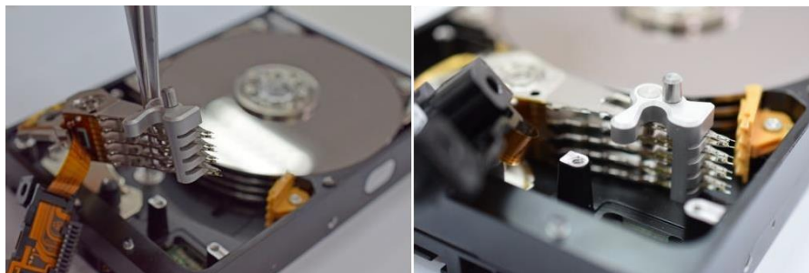
Picture 6.12 Mounting the heads on the patient drive and moving them to the ramp
