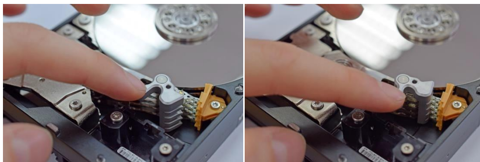
Picture 6.6 Rotating the tool - snouts are positioned between the heads
