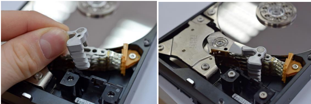
Picture 6.5 Mounting the tool on the actuator arm
