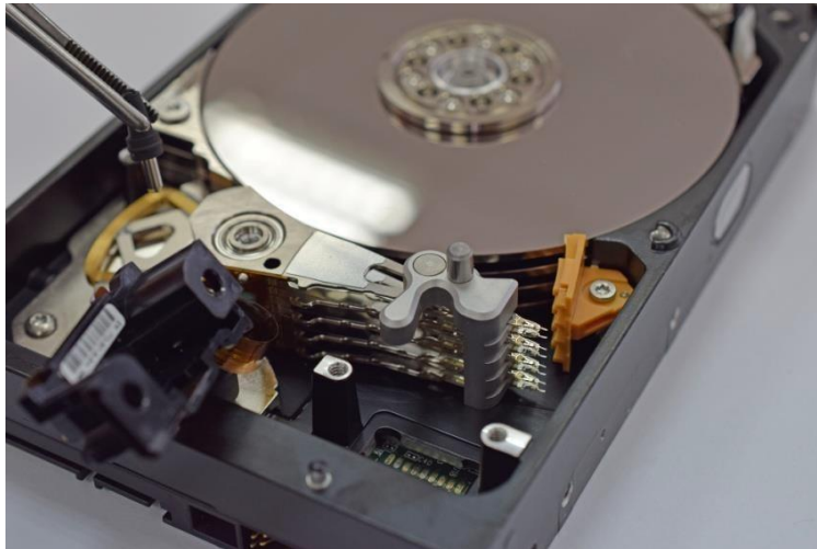
Picture 6.9 Removing the security brake
