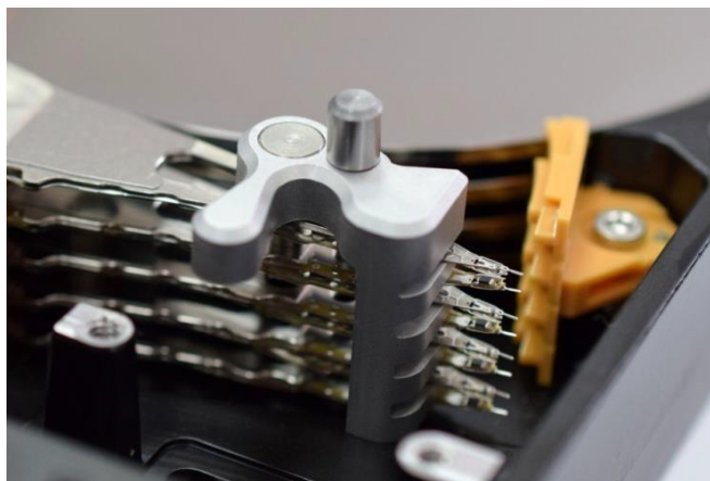
Picture 6.10 Sliding the heads off the donor drive ramp
