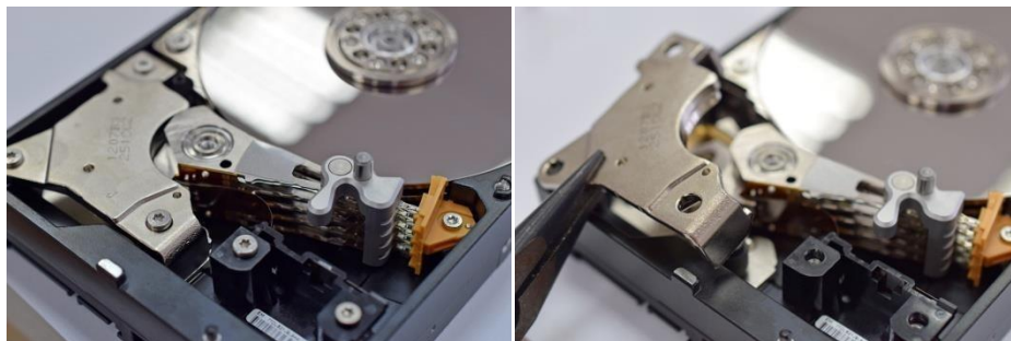
Picture 6.8 Removing the screws connecting upper magnet to the HDD casing (left); Removing the upper magnet with the needle-nose pliers (right);
